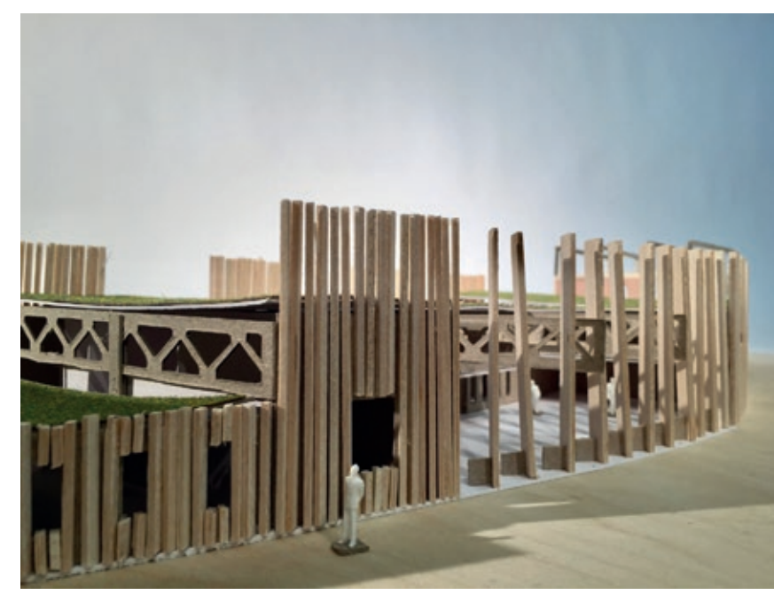
The wood cladding, that runs across the whole main section of the building is manipulated to create openings for windows and views into and out of the large void which is used as an exterior extension of the daycare.
