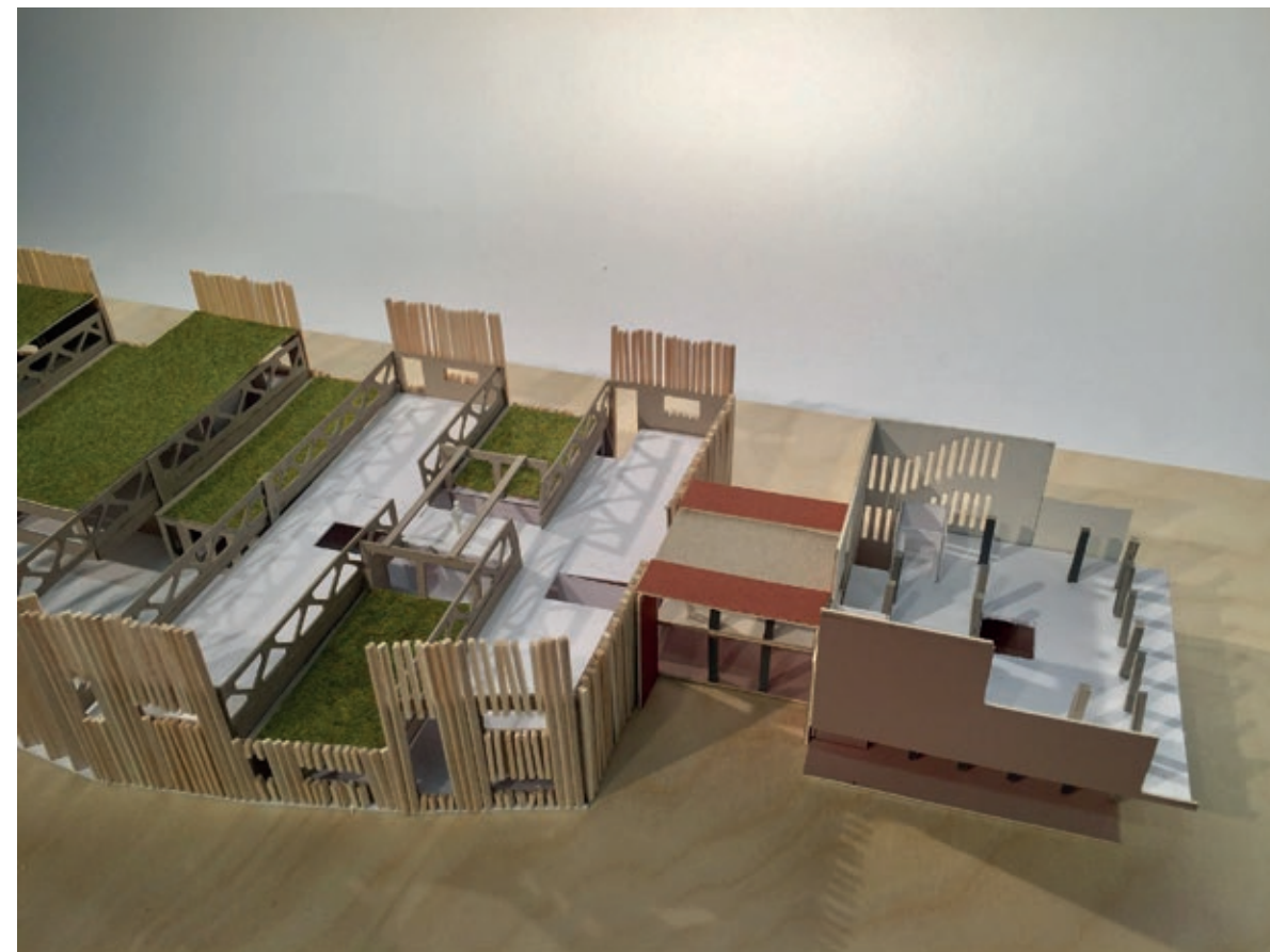
The first floor of the creative hub spanning across the two part of the building and the walkway that cuts through two structural trusses supported by extra columns below.
