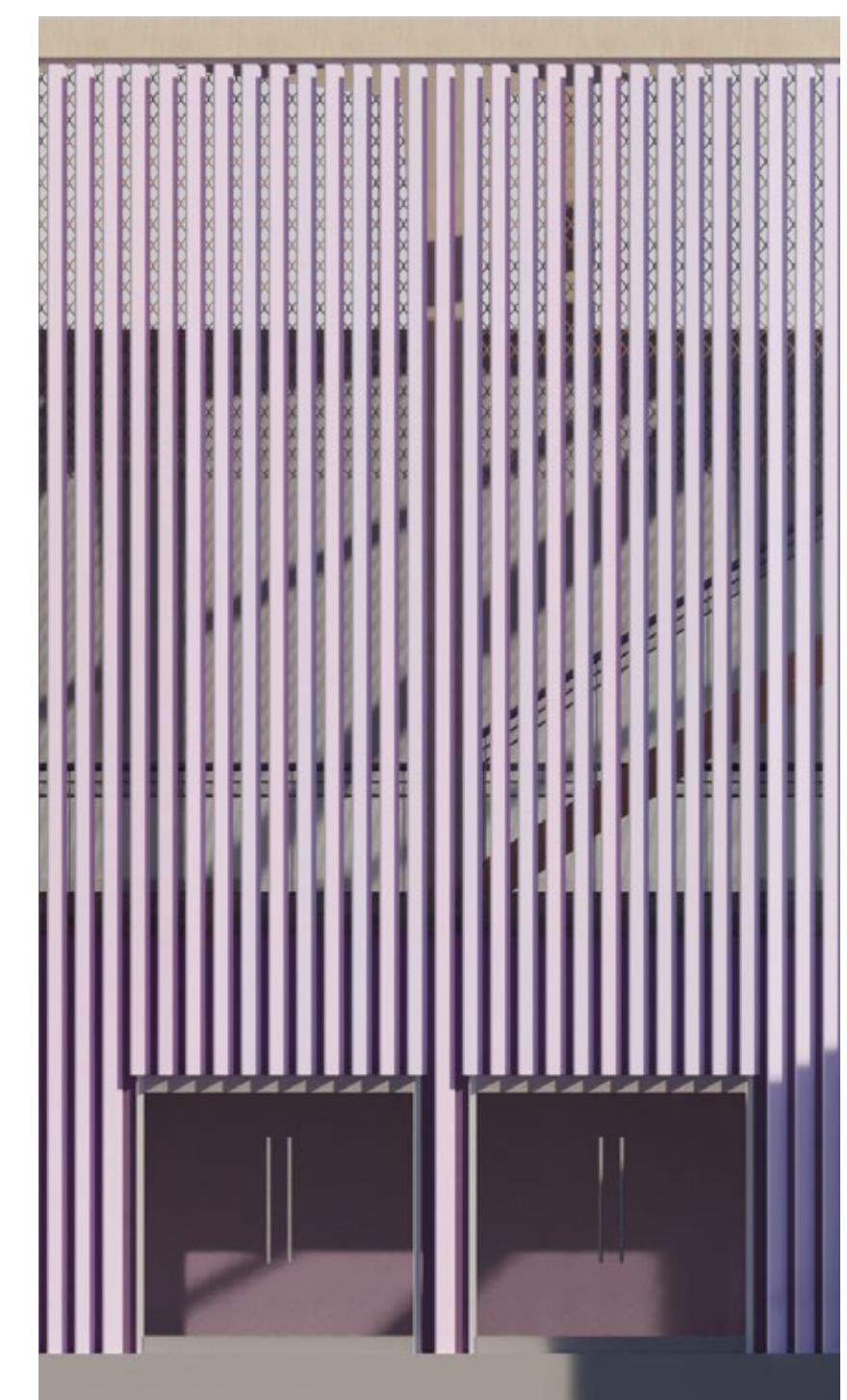
Louvers closed to minimize solar gain and stop overheating. Allows for more private spaces as the 'insides' of building are hidden.
