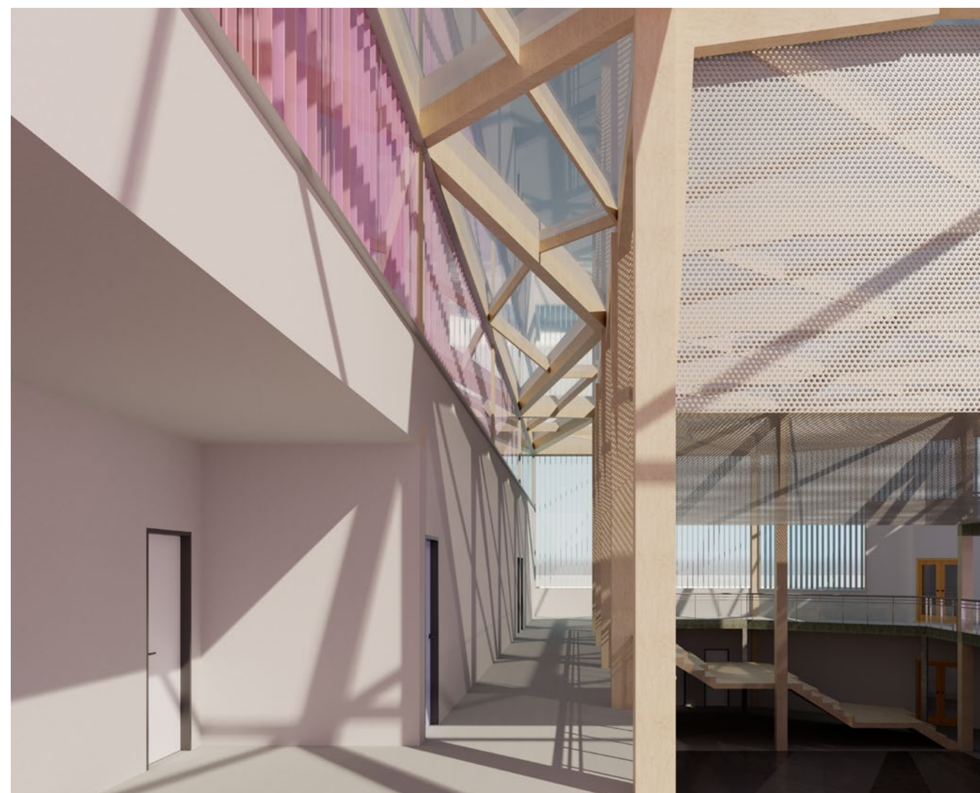
The hallway under normal lighting conditions, leading to harsh shadows, a lot of solar gain and most likely overheating that can't be resolved by natural ventilation.
